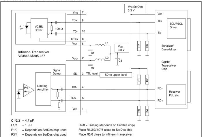
Values of R1/2/3/4 may vary as long as proper 50  $\Omega$  termination to V<sub>EE</sub> or 100  $\Omega$  differential is provided. The power supply filtering is required for good EMI performance. Use short tracks from the inductor L1/L2 to the module V<sub>CC</sub>Rx/V<sub>CC</sub>Tx.
