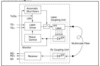
The receiver component converts the optical serial data into PECL compatible electrical data (RD and RDnot). The Signal Detect (SD, active high) shows whether an optical signal is present.
