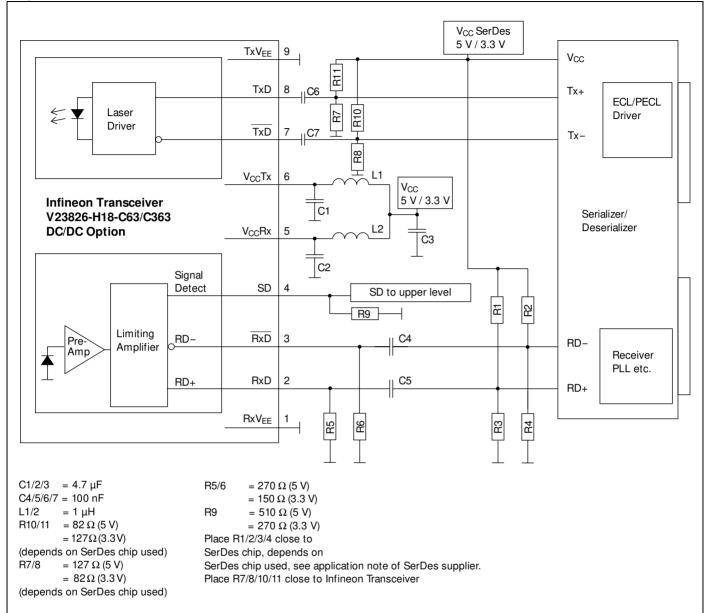
This Application Note assumes Fiber Optic Transceivers using 5 V power supply and SerDes Chips using 3.3 V power supply. It also assumes no self biasing at the receiver data inputs (RD+/RD-) of the SerDes chip (Refer to the manufacturer data sheet for other applications).
