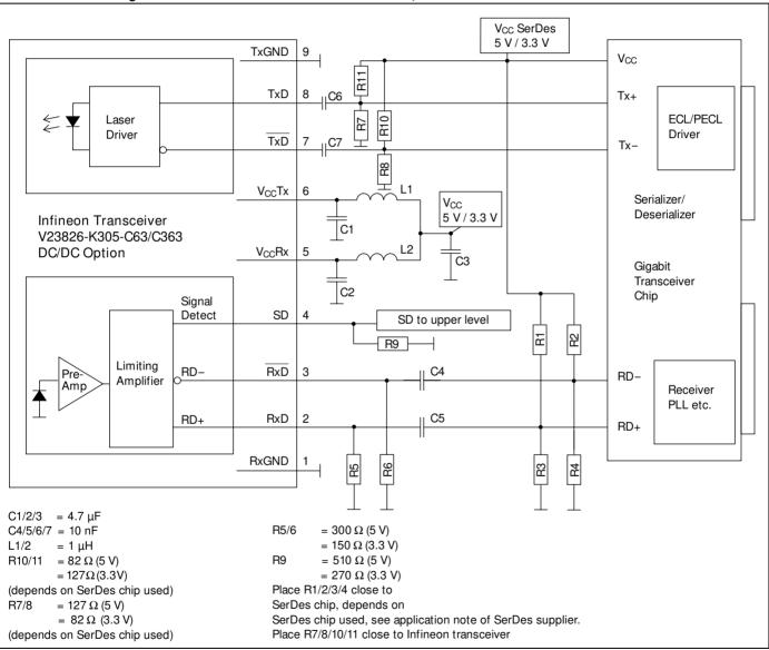
This Application Note assumes Fiber Optic Transceivers using 5 V power supply and SerDes Chips using 3.3 V power supply. It also assumes self biasing at the receiver data inputs (RD+/RD-) of the SerDes chip. Refer to the manufacturer data sheet for other applications. 3.3 V-Transceivers can be directly connected to SerDes-Chips using standard PECL Termination network.
