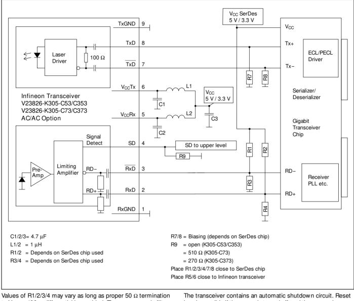
Values of R1/2/3/4 may vary as long as proper 50  $\Omega$  termination to V<sub>EE</sub> or 100  $\Omega$  differential is provided. The power supply filtering is required for good EMI performance. Use short tracks from the inductor L1/L2 to the module V<sub>CC</sub>Rx/V<sub>CC</sub>Tx.
