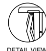
DETAIL VIEW VH1, VH3 & VH5 HOLE PLUGS (No wing serrations for ease of removal)
