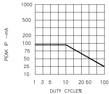
Fig.5 MAX PEAK CURRENT VS. DUTY CYCLE % (REFRESH RATE f=1KHz)
