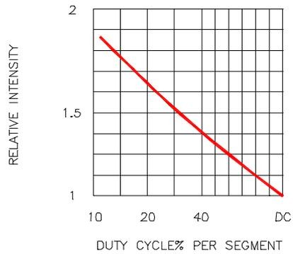
Fig.4 LUMINOUS INTENSITY VS. DUTY CYCLE
