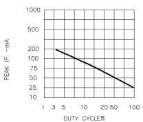
Fig.6 MAX PEAK CURRENT VS. DUTY CYCLE %
