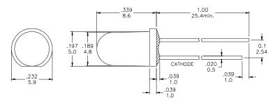
Unit: ± inch/mm \*Tolerance:  $\pm \frac{0.01}{0.25}$
