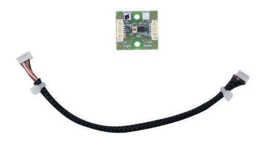
UDOO Bricks are modules you can use to augment your UDOO boards and make them more versatile. Attach them into I2C snap-in connector with the related cable. UDOO Bricks work along a cascade configuration, so you can attach them all together without wasting space in a truly intuitive way. Thanks to such configuration you can use cables up to 3,5 m long to connect UDOO Bricks one another.
