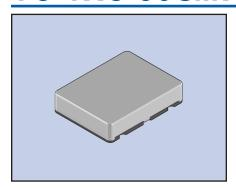
The VC-TXO-39SMX is a VC (Voltage Controlled) **FEATURES** TCXO (Temperature Compensated Crystal Oscillator) featuring very tight stability over a wide temperature range. The small SMD ceramic package measures 11.4 x 9.6 x 2.3 mm. The voltage control has a tuning range of  $\pm$  12 ppm typical. The low profile package is ideal for wireless communications applications.
