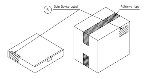
Type A Material / box : Cardboard C5BF Type B,C Material / box : Cardboard K5AF Partition : Cardboard K5BF
