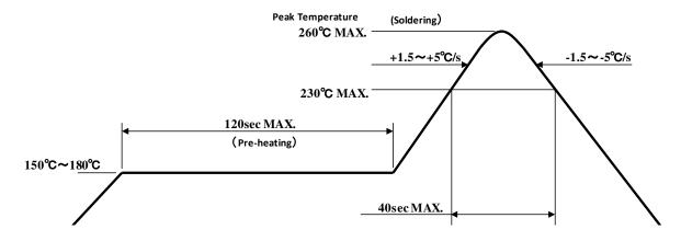
Note 1 Temperature Profile for the reflow should be set to the surface temperature of resin which is on the top of LED. This should be the maximum temperature for soldering. Lowering the heating temperature and decreasing heating time is very effective in achieving higher reliability.
