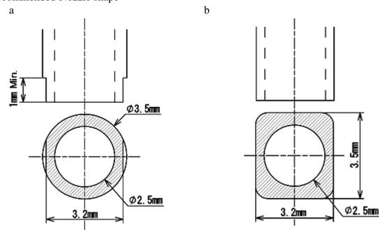
\*Nozzle with chamfering is recommended
