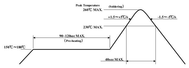
Notes 1 Recommended temperature profile for the reflow soldering is listed as the temperature of the resin surface. This should be the maximum temperature for soldering. Lowering the heating temperature and decreasing heating time is very effective in achieving higher reliability.
