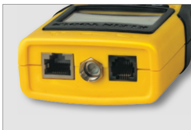
Top View: RJ45, RJ11/12 and F-connector ports
