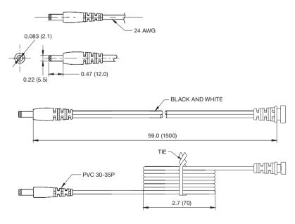
Wire type: VW-1 80°C 300 V L=1500 mm 2464 20 AWG for 5 V output, 22 AWG for 9 V ouput, 24 AWG for 12 V output, 2C Black and White. Black - Negative, White - Positive
