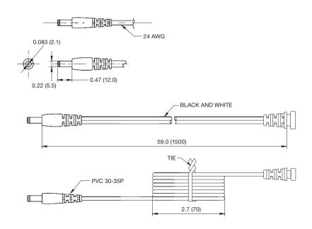
Wire type: VW-1 80°C 300 V L=1500 mm 2464, 18 AWG for 12 V output, 20 AWG for 15 V ouput, 22 AWG for 18 and 24 V output, 2C Black and White. Black - Negative, White - Positive
