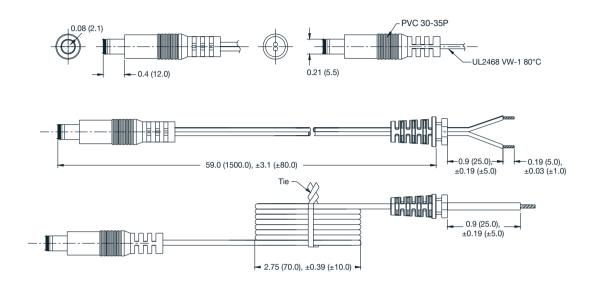
Wire type: VW-1 80°C 300 V L=1500 mm 2464 18 AWG for 12 V output, 20 AWG for 15 V ouput, 22 AWG for 18 and 24 V output, 2C Black and White. Black - Negative, White - Positive
