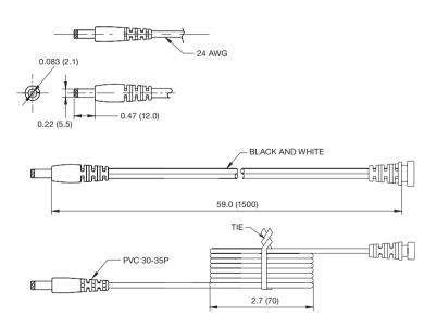
Wire type: VW-1 80°C 300 V L=1500 mm 2468, 18 AWG for 12 V output, 20 AWG for 15 V ouput, 22 AWG for 18 and 24 V output, 2C Black and White. Black - Negative, White - Positive
