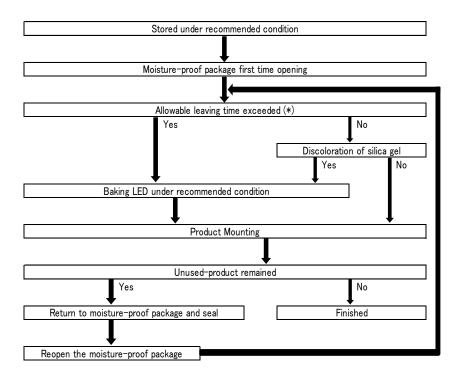
Allowable leaving time means the maximum allowable leaving time after opening package, which depends on each LED type.
