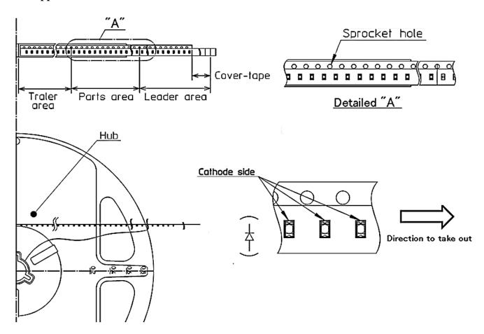
Note "-TR" means cathode side of LEDs should be placed on the sprocket-hole side.
