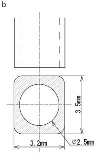
\* Nozzle with chamfering is recommended
