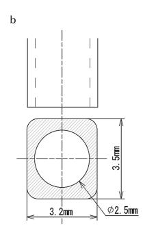
\* Nozzle with chamfering is recommended
