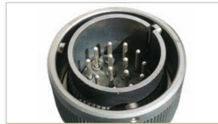
Cannon designed insulators are manufactured from high quality polychloroprene to withstand temperatures from -55C to +125C (-67F to +257F) and provide sealing in the unmated condition.
