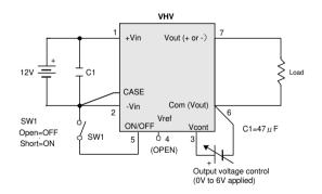
The VHV series does not basically require additional parts, but add capacitor C1 to the input terminal if input impedance is high due to a long distance between the power supply and converter, the input line is thin, a filter is inserted on the input side, etc. When fitting a capacitor, try to add on the converter terminal side so as to reduce lead inductance.
