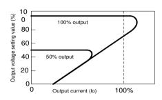
The overcurrent protection circuit shows a drooping characteristic. Ensure that the load to be used is at least with the minimum resistance specified for each series.
