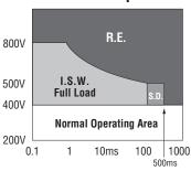
I.S.W.: Input surge withstand, no degradation of performance. R.E.: Ratings Exceeded S.D.: Shutdown
