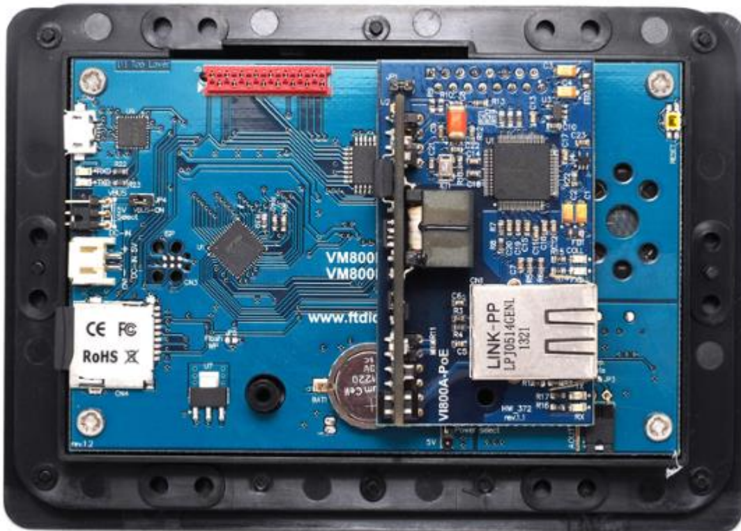
Figure 5-1 – VI800A-PoE module connected to VM800P Plus module
