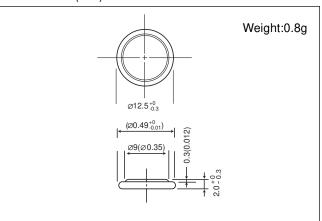
**Note:** This bare cell diagram is for size reference only. Please refer to the tab configurations at the end of this section for available tabs.
