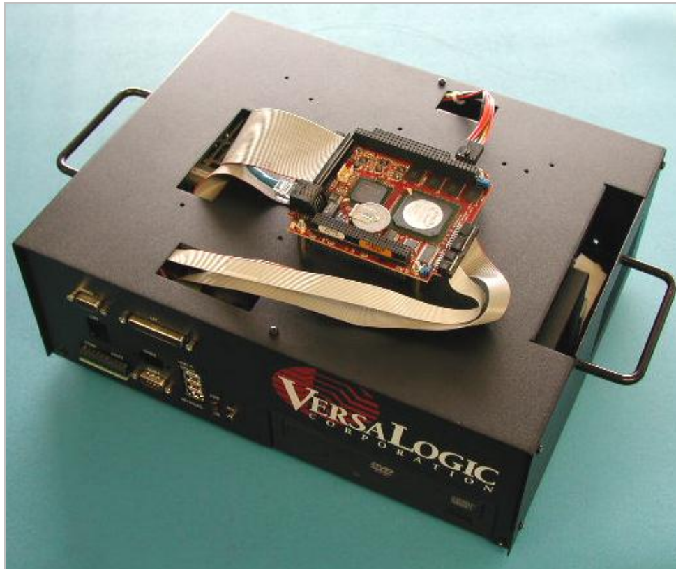
Figure 9. Example PC/104 Board Installation
