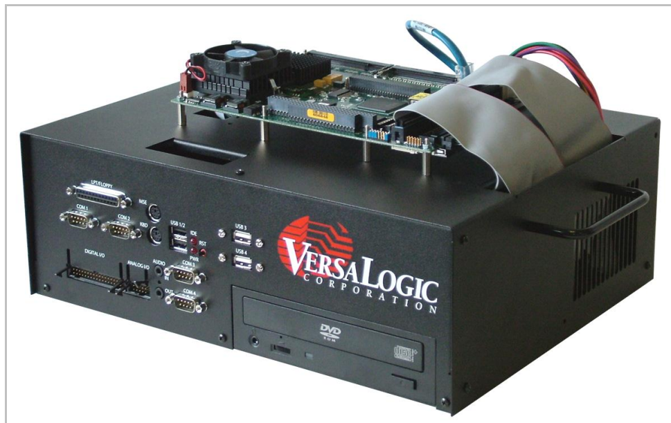
Figure 10. Example EBX Board Installation
