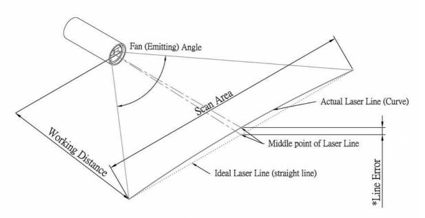
\*Laser Line Accuracy =  $\frac{\text{Line Error at middle point}}{\text{Scan Area}}$ For VLM-650-30 Series, Laser line accuracy <  $\frac{4}{1000}$
