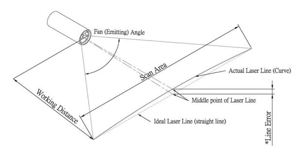
\*Laser Line Accuracy =  $\frac{\text{Line Error at middle point}}{\text{Scan Area}}$ For VLM-650-30 Series, Laser line accuracy <  $\frac{4}{1000}$ For VLM-650-41 Series, Laser line accuracy <  $\frac{1}{100}$
