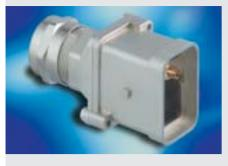
Cable connectors for female contact inserts, for cable diameter 8 - 23 mm and wire sizes 0.5 - 10 mm², 20 - 8 AWG. For contacts see page 7.
