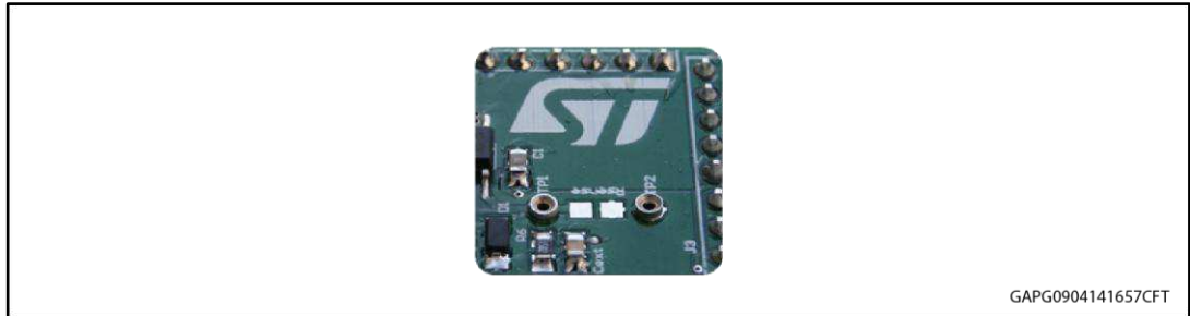
Figure 4: Mounting through-hole sense resistor
