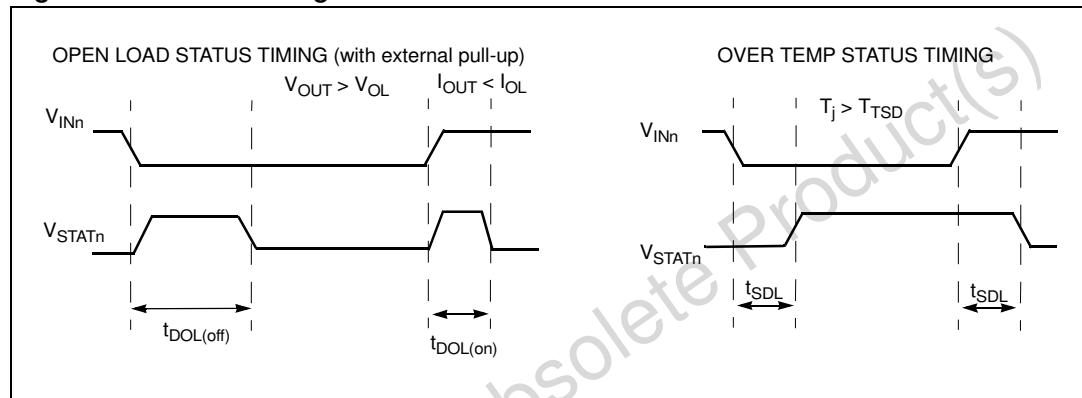
**Figure 5. Switching time waveforms**
