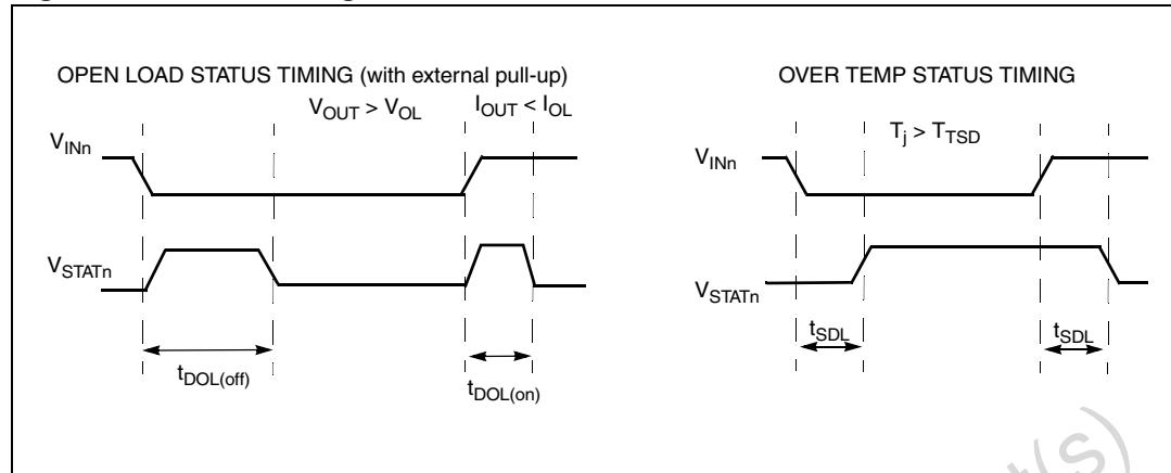
**Figure 5. Switching characteristics**
