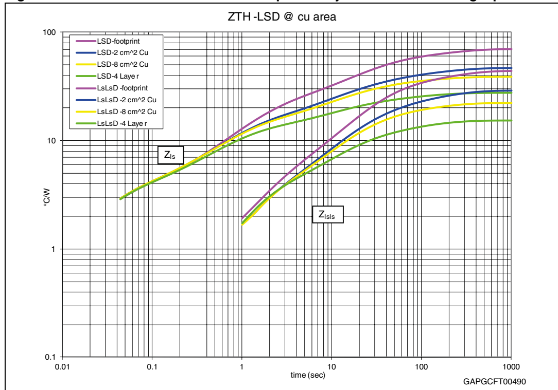
Figure 16. PowerSSO-36 LSD thermal impedance junction ambient single pulse
