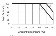
① Convection 2 Forced air (0.5m³/min) (18 CFM)
