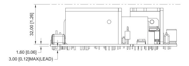
1. CN1 mates with Molex housing 09-50-3031 with Molex 2478 series crimp contact or equivalent. Notes:
