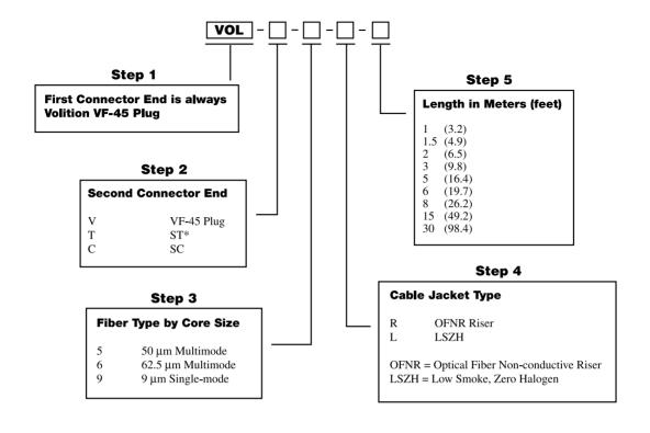
Example: VF-45 to ST\*, 9 µm Single-mode OFNR Cable, 2 meters.
