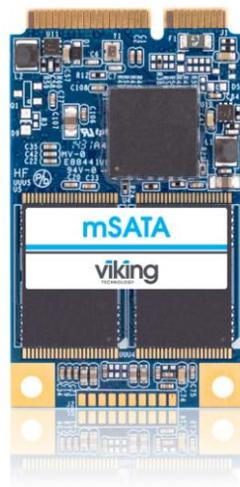
mSATA (mini-SATA, MO-300) is a non-volatile, solid-state storage device delivering Serial ATA performance, reliability and ruggedness for industrial and environmentally challenging applications.
