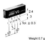
Pin Grid 2.54 PCB hole dia 0.6
