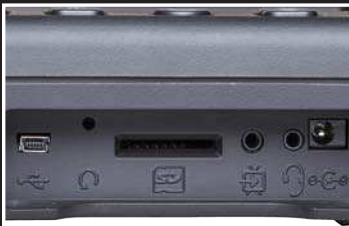
Inputs include USB port, SD card slot, video out, earphone and AC power jacks
