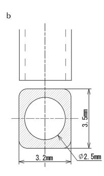
\* Nozzle with chamfering is recommended
