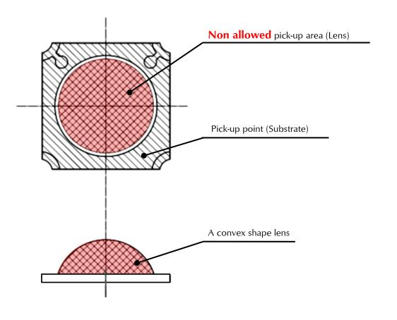
Please adjust the load, pick-up point, nozzle diameter, etc. before mounting because over load can cause breakage of the product.
