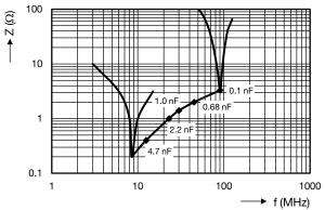
Lead configuration: length = 30 mm, lead spacing: standard, lead diameter: standard, inline crimp
