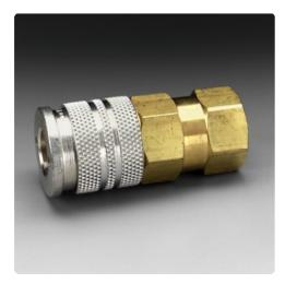
This socket is a high pressure hose socket that may be used on the  $3M^{\text{TM}}$  Supplied Air Hose W-9435 and W-2929. It is a 1/4 inch FPT brass fitting.
