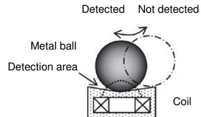
\*4. Whether the metal ball built in the sensor is detected or not determines the ON/OFF state of the output transistor. (Intermittent output)
