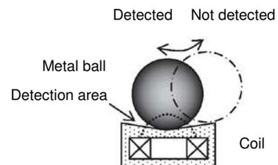
\*4. Whether the metal ball built in the sensor is detected or not determines the ON/OFF state of the output transistor. (Intermittent output)
