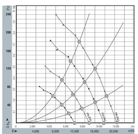
Air performance measured as per: ISO 5801, Installation category A, in ebm-papst full nozzle and without protection against accidental contact.
