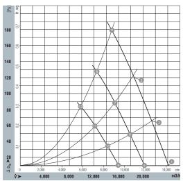
Air performance measured as per: ISO 5801, Installation category A, in ebm-papst full nozzle and without protection against accidental contact.
