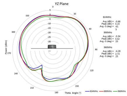
GSM antenna High band Radiation Pattern X-Y Plane\*
