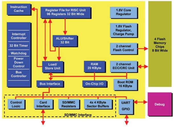
Figure 1: Card Block Diagram
